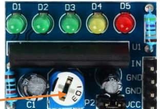
The sensitivity of the movement is controlled by the Potentiometer located on the KA2284 board. You will have to fiddle with it based on the loudness of your MP3s.
